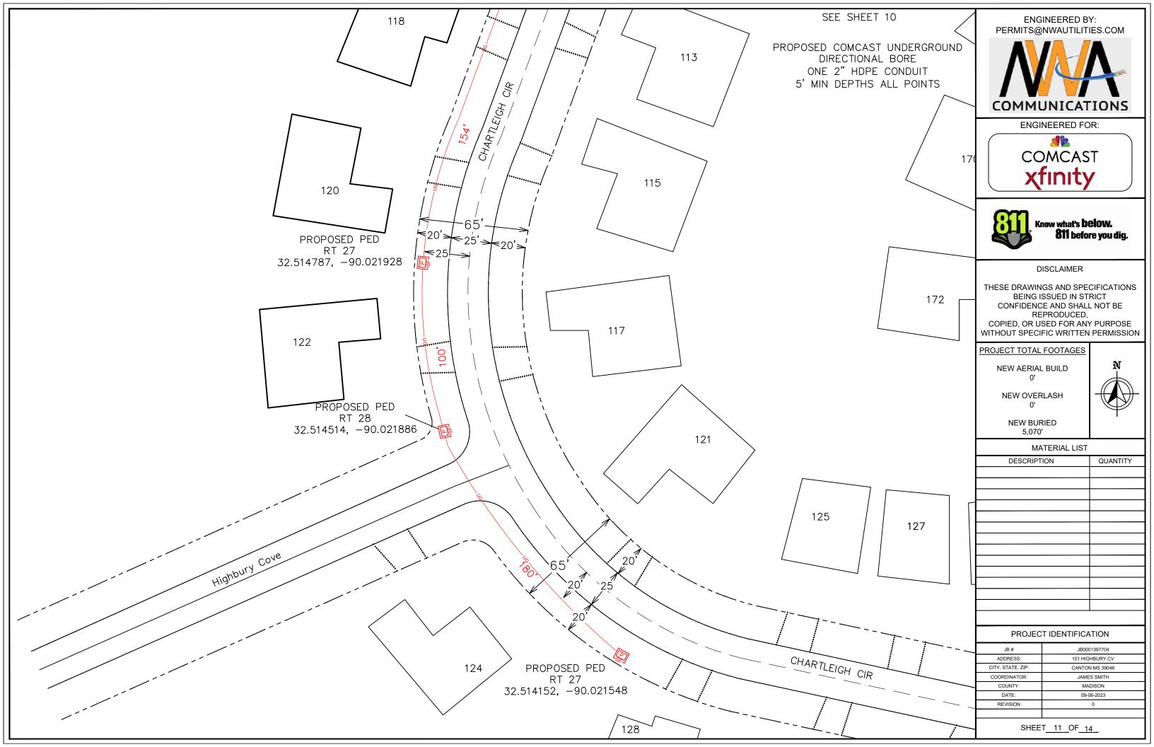
PROPOSED COMCAST UNDERGROUND DIRECTIONAL BORE ONE 2" HDPE CONDUIT 5' MIN DEPTHS ALL POINTS
